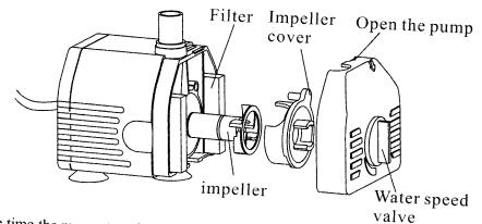
If after some time the pump starts losing power or stops working you should check for the build up of sediment or scale in the filter or in the pump housing. The filter housing can be remover by pressing down on the bottom of the filter housing.
